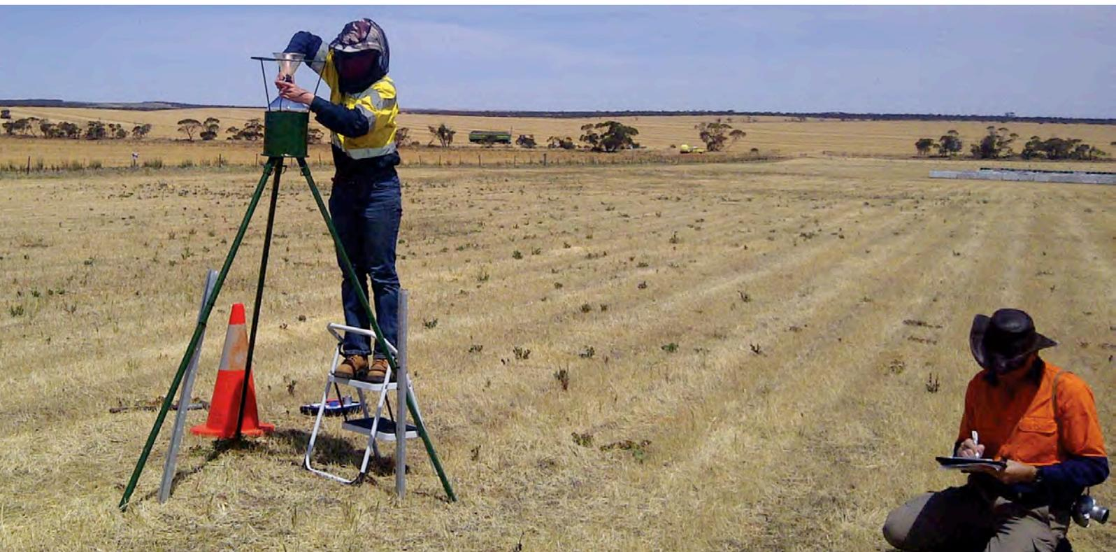
*Collection from dust deposition gauge near proposed mine site at Warrambo*
