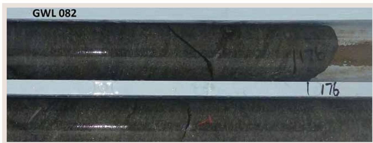
Figure 22: Typical mineralised PQ core from metallurgical drill hole GWL082
