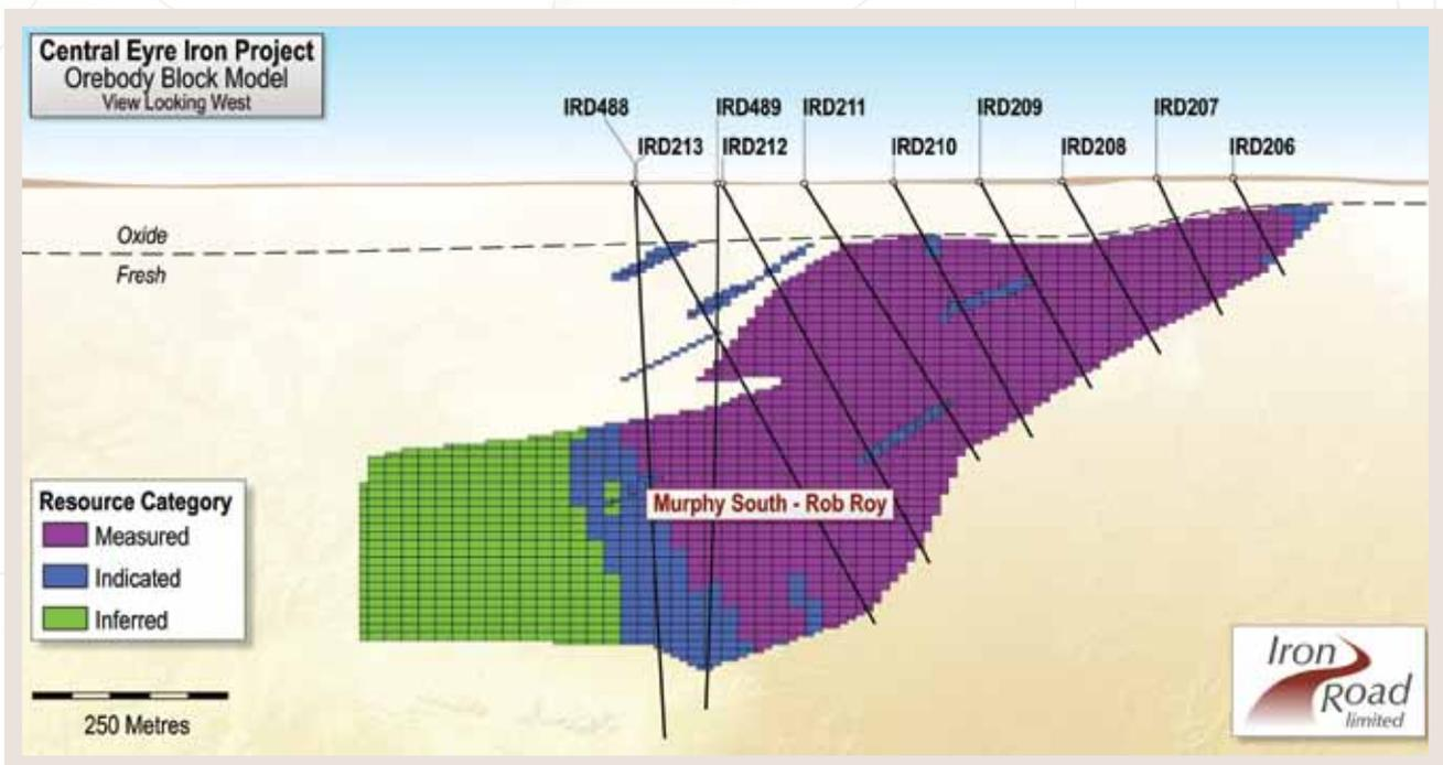
Figure 7: Cross section through the Murphy South - Rob Roy area of the Warrambo Resource block model
