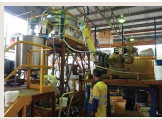
Figure 14: Pilot milling circuit in operation at Amdel. The mill is located within the yellow guarding in centre right of the picture.
