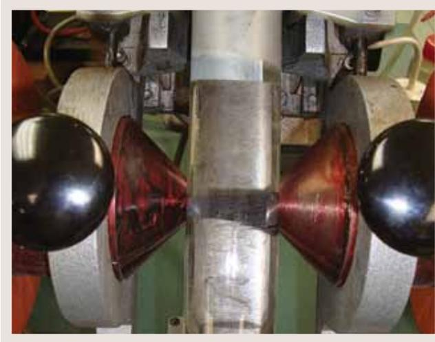
Figure 12: Davis Tube Recovery Test apparatus. Magnetite concentrate is suspended between the two magnetic poles.
