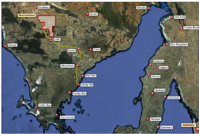
Figure 6 – Concentrate pipeline route
