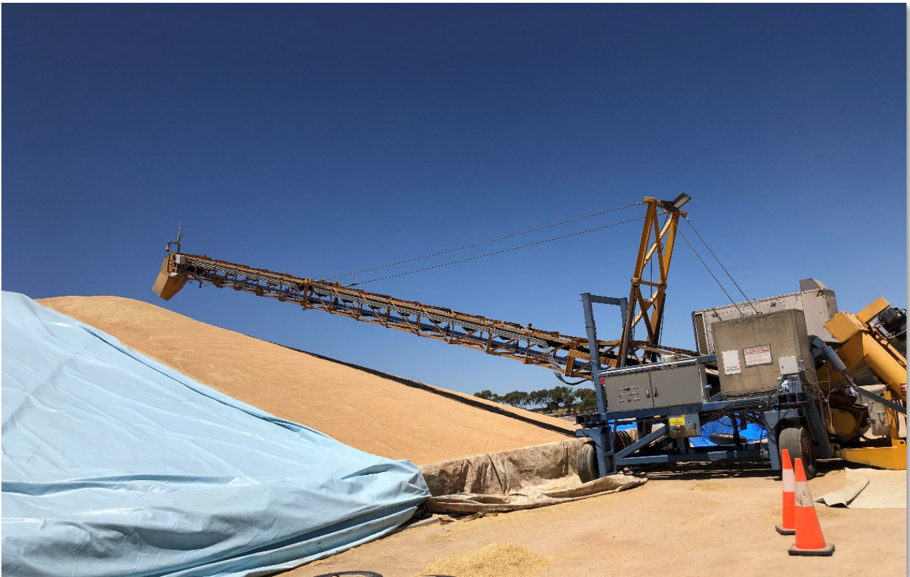
Horizontal bunkers will be fitted with a traditional tarpaulin cover arrangement
